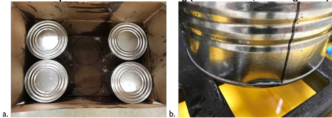
Picture 7: Option 3 after vibration testing (a. stained box, b. damaged can)
